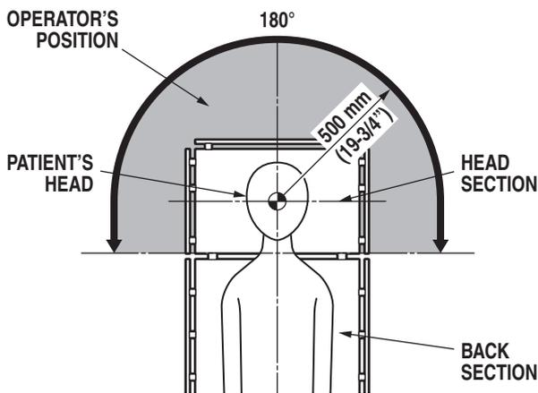
Figure 2-5. Operator's Position
