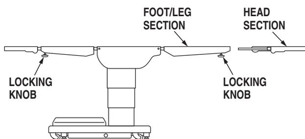
**Figure 2-22. Repositioning Head Section
