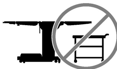
Do not place objects on the base of the table, a danger of damage exists during positioning.
