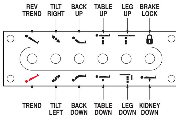
Figure 2-19. Emergency Back-Up Controls
