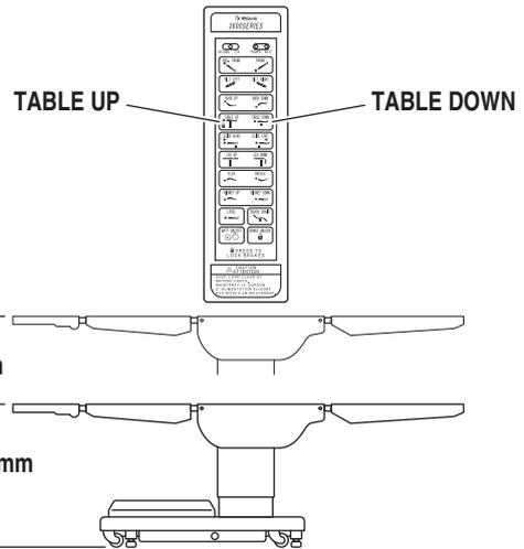
**Figure 2-10. Elevation Function**
