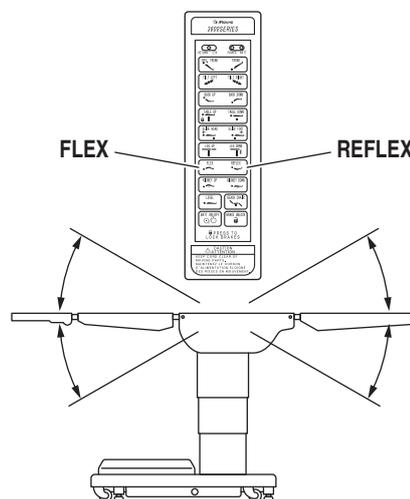
Figure 2-13. Flex/Reflex Positioning
