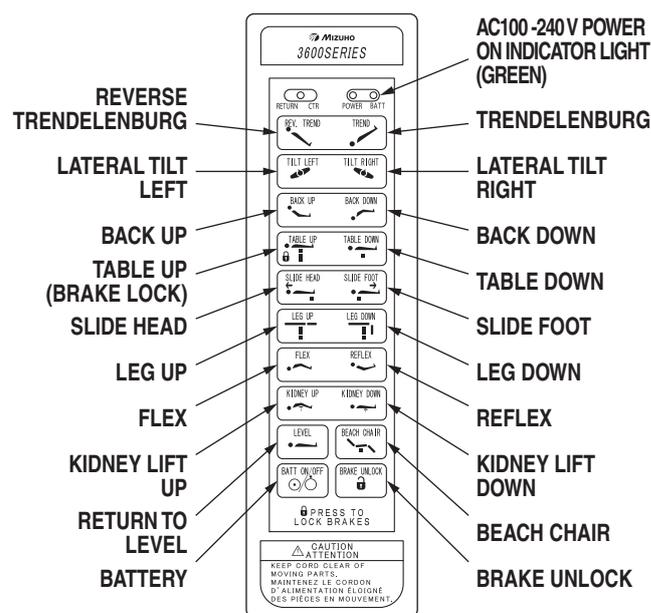
Figure 2-4. Pendant Control Function Buttons
