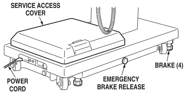
Figure 2-20. Emergency Brake Release
