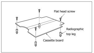
Attach the radiographic top legs to the cassette board with the flat head screws.
