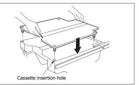
Align the end of the radiographic top legs to the cassette insertion holes of the tabletop and insert the cassette board straightly.
