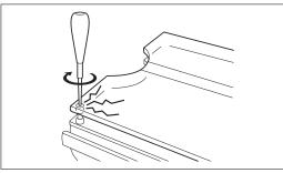
1-6. Do not detach as shown below. It could damage the cassette board.
