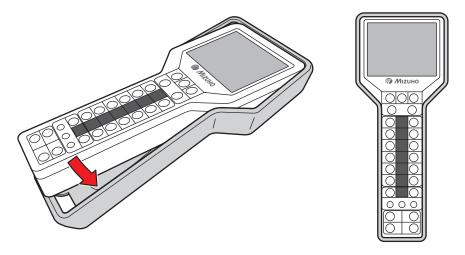
3. Align the connector with the guide and insert it into the receptacle properly.
