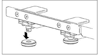
Note: If an accessory interferes with the fixing handles, the fixing handles can be detached by pulling them downwards.
