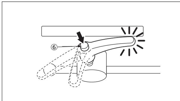
In case the adjusting lever contacting with the board and interfere with the operation, move the adjusting lever with the button⑥ pushed down.
