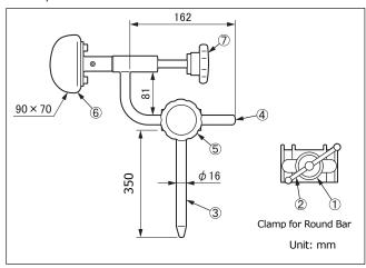
Note: The rail clamp shown above is Clamp for Round Bar.
