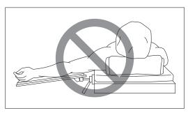
Do not use this product if its upper surface is lower than the surface of the operating table.
