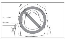
Do not use this product together with the shoulder support for a patient in the Trendelenburg position (laid flat on the back with the feet higher than the head). (Refer to the Interactions section.)
