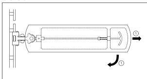
Pull the rotation lever to rotate the armboard up to 90 degrees.
