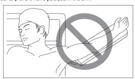
Do not allow the arm to be positioned at an angle of more than 90 degrees with respect to the longitudinal direction of the operating table.
