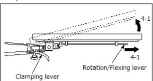
4-1 After pulling the rotation/flexing lever, the arm board can be flexed up to 15 degrees.
