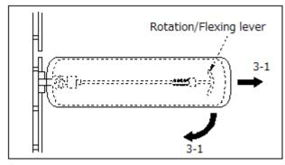
3-1 After pulling the rotation/flexing lever, the arm board can be rotated up to 90 degrees.
