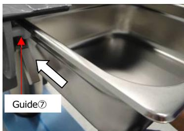
1-4. Pull the uro drain tray<sup>①</sup> toward you to check that the stopper works to prevent the uro drain tray<sup>①</sup> from coming off.
