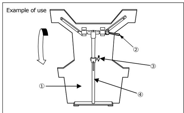
Use the folding lever② to put the support pole④ into the storage position.
